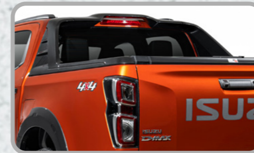
CENTRE HIGH MOUNTED STOP LAMP: Complete with emergency stop signal, this new feature significantly enhances vehicle visibility.
