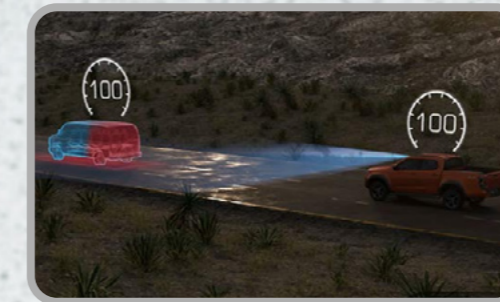
ADAPTIVE CRUISE CONTROL [ACC]: Your ISUZU D-MAX ARCTIC TRUCKS AT35 automatically maintains a pre-set speed and distance from the vehicle ahead. Stop-and-go functionality keeps ACC settings active for up to five minutes when stopped.
