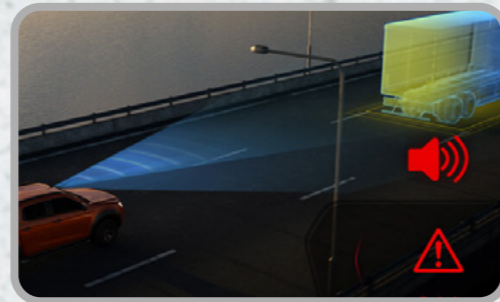
AUTONOMOUS EMERGENCY BRAKING [AEB]: Your ISUZU D-MAX ARCTIC TRUCKS AT35 features automatic emergency braking, activated on detection of a potential frontal collision.
